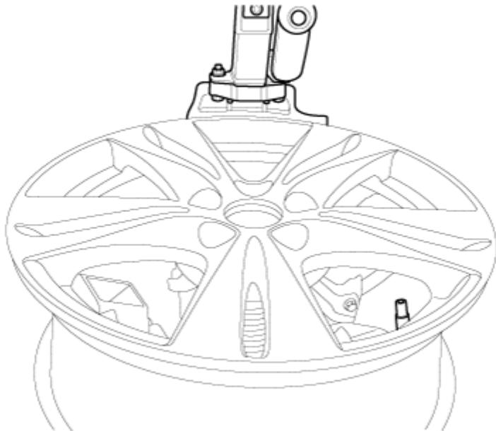
3. Place the tire on the rim so the bottom bead touches the edge of the rim after the valve (6 o'clock). Rotate the rim clockwise, and push down on the tire at the 3 o'clock position to fit bottom bead.
